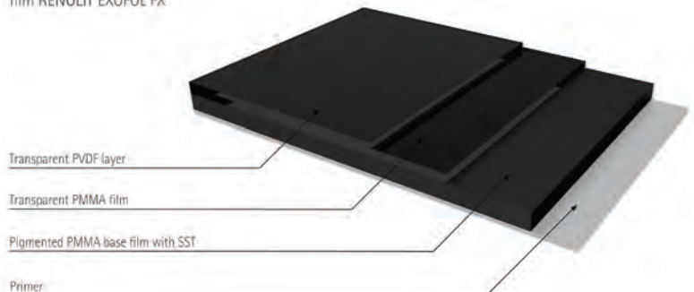
Diagram showing the structure of the exterior film RENOLIT EXOFOL FX
